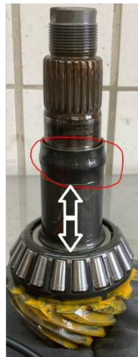
This one does have a crush spacer on it, circled in red.
