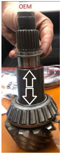
This one does not have a crush spacer on it.
