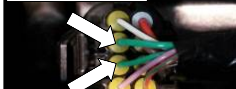
Small Green wire (do not connect to this)
