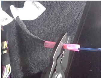
29. On the vehicle left hand side footwell, locate vehicle wire with label "RUN START".
