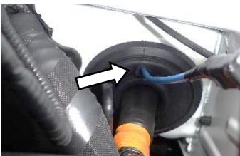
27. Spray the pipe and taped "VEHICLE IGNITION" wire with lubricant.
