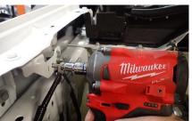
45. Locate the TAPTITE thread forming screw as shown.
