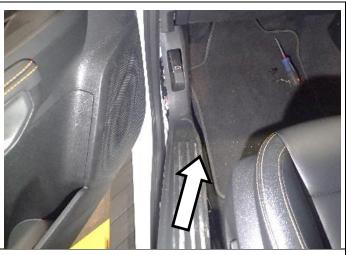
20. Remove door sill panel as shown. This can be removed by lifting the sill panel and then rotating up.
