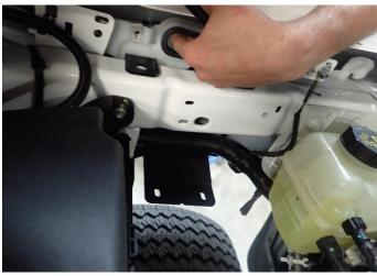
Loosen the two earth ring terminals to allow battery tray to be fitted onto the hydroform.
