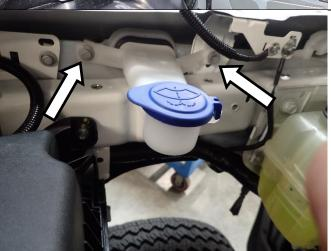
22. Remove washer bottle filler neck by undoing the two fasteners shown.
