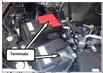
Locate the main battery and disconnect both terminals, beginning with the negative.
