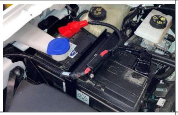
50. Fasten the 40A fuse holder to the battery clamp using the M4 fasteners provided and route cables appropriately using cable ties.
