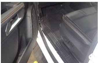
19. Lift the rubber seal surrounding the left hand side sill panel.
