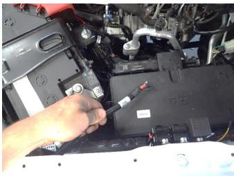
9. Pull out "START BATTERY" wire to behind battery.
