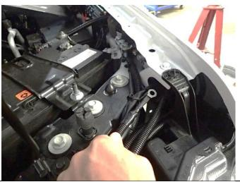
36. Route "ANDERSON PLUG GROUND CABLE" ring terminal through gap behind quarter panel support.
