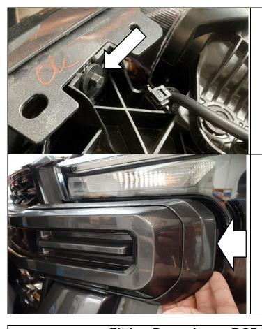
17. Remove the top two bolts which secure the grille.
