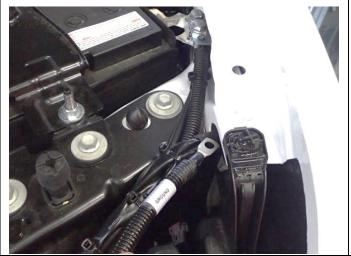
4. Source M8 bolt and nut, fit bolt into "GROUND" terminal.
