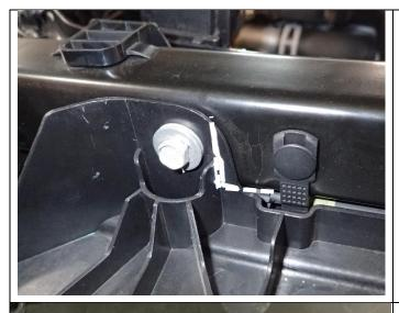
4. Mark the following items on the radiator trim panel as shown and trim with sidecutters or an oscillating multi-tool.
