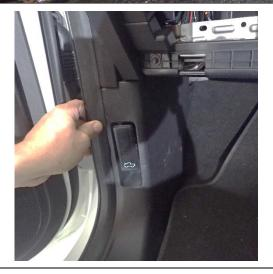
31. Refit the passenger side footwell panel. Press at various locations to ensure all clips are engaged.
