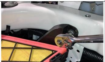
Gently maneuver the air box upwards so that the two locating pins are freed from their rubber housings. Place air box to the side safely.
