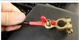
48. On the "AUXILIARY BATTERY POSITIVE CABLE", push the ring terminal into the red terminal cover.
