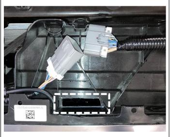
6. Cut four cable ties holding the loom at the points shown.
