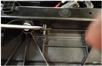
9. Drill a Ø 10mm hole in the radiator cover panel in the position shown.
