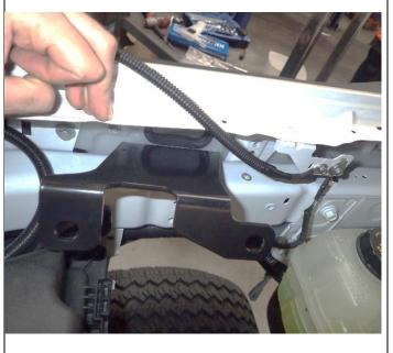
28. Place the battery support bracket onto the vehicle rail.
