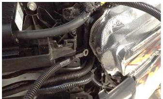
35. Route "ANDERSON PLUG GROUND CABLE" ring terminal though gap to behind headlight.
