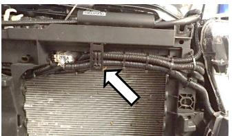
40. Beneath the radiator trim panel, secure harness bundle with cable ties.
