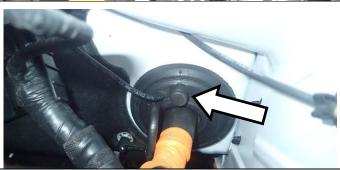
21. Locate firewall grommet located in the engine bay behind the left hand side fuse box.
