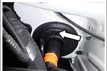
22. With a sharp blade, cut and remove the nipple from the firewall grommet.
