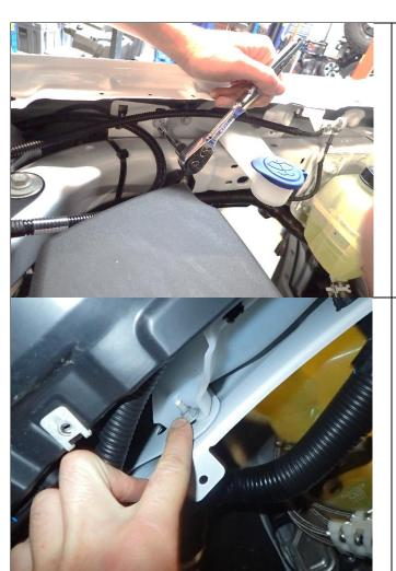
26. Loosen and temporarily remove the water bottle fastener shown. Set aside fastener to be refitted later.
