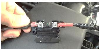
17. Install the AUXILIARY BATTERY POSITIVE CABLE M5 ring terminal onto the AUXILIARY MIDI FUSE.
