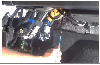
28. On the vehicle left hand side footwell, locate and pull the pipe through the firewall grommet.
