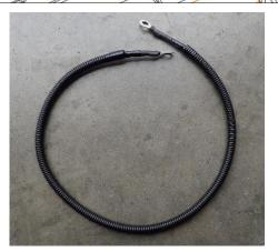
44. Locate the "AUXILIARY BATTERY GROUND CABLE" with M8 ring terminals on each end as shown.
