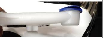
Refit the washer bottle stem using the fasteners previously removed in Step 22.
