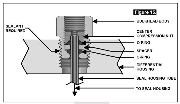
NOTE: Make sure the seal housing tube is all of the way into the center compression nut while you are tightening it.
