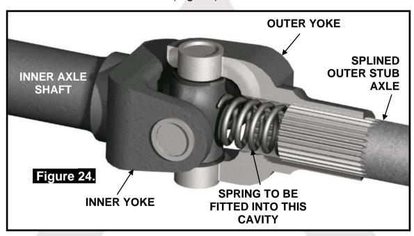
When assembled, ensure that the spring maintains sufficient pressure on the axle to hold it firmly against the cross shaft of the differential while the vehicle is sitting on level ground.
