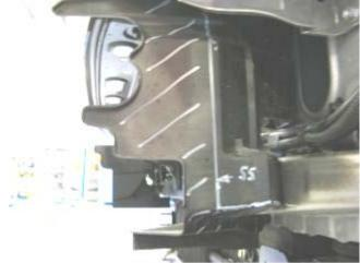
40. Mark out and trim the air deflector on the LHS of the vehicle using a pair of tin snips or similar.
