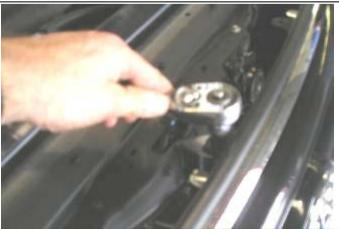
8. Remove 3 X retaining screws from top of grille
