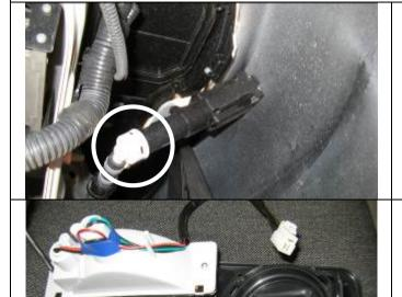
81. If headlight cleaner system to be fitted, reconnect circuit at main joint to vehicle and also hoses to tails of spray heads
