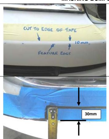
Apply wide masking tape edge, carefully aligning 10mm above bumper feature line as shown. Keep the same line level through the centre section of the bumper as shown
