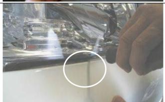
21. Push bumper down immediately below headlamp to gain access with a small flat blade screwdriver and release holding tab.
