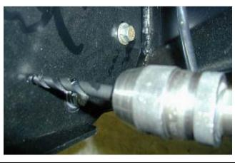
80. With access through light aperture in wing, using the M10 pilot holes in mount brackets (located up 175mm from bottom face of bar), drill pinning hole through uprights on bull bar. Fit M10 screw, washer set and flange nut and do up tight.
