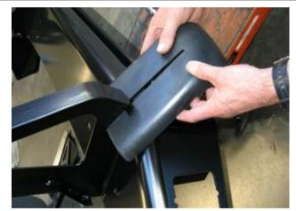
64. Carefully slide top section of buffer past edge of cover strap as shown
