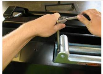
56. Fit the roller fair lead, pull only the end of the cable through and adjust the position of winch then bolt up securely. Use the 1 ½" long bolts in the top and 1 ¾"in the lower set through the RFL.
