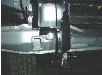
8. Fit M10 SEMS bolt and load flange nut from inside cross member then do up tight.
