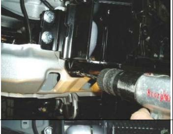
Drill Dia 10.5 pinning hole in lower flange of mount bracket into the vehicle crossmember
