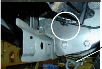
9. With the out board bracket in position and bolted securely (as shown) re-clip the electrical loom connector. The flange on the top of the bracket is to house the connector and snaps into place.
