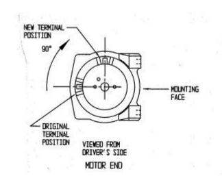
12. To place the winch motor in the correct location the winch motor must be rotated 90 degrees, in a clockwise direction when viewed from the motor end.
