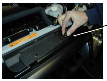
With all of the plastic plugs, two screws and two bolts removed from the lower bumper bar, the grille and grille cover must be removed. There are three plastic plugs that hold the cover in place, remove these as previously described above.
