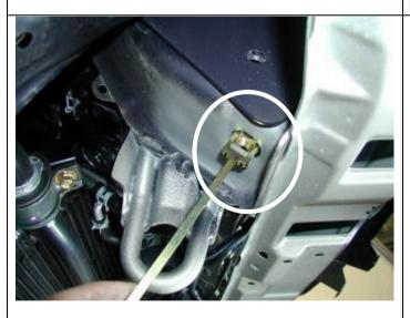
4. The three bolts that hold the washer bottle need to be removed to provide clear access to the chassis.
