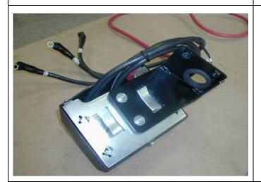
8. Fit the control box bracket to the control box using the 4 large M6 flat washers placed either side of the bracket and secure using the original 1/4" nuts. Finger tighten only at this stage.
