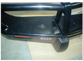
11. When the control box is secured to the bull bar, adjust the control box so that the remote cap is central in the cutout in the wing. When satisfied tighten the control box to control box bracket bolts and the control box bracket to bull bar bolts.
