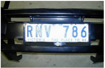
5. If a winch is not being fitted place double sided tape across the back of the number plate and fix in place to the lower holes in the bull bar using 2 M6 x 20mm bolts, M6 flat washers and M6 flange nuts.
