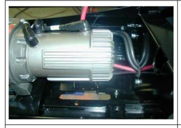
15. Connect the winch control box cables to the winch. Refer to the Warn installation instruction manual when wiring up winch.
