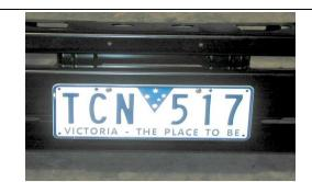
111. Fit the plastic plugs into the square holes in the lower pan. Fit the number plate to the bull bar using the black self-tapping screws.
