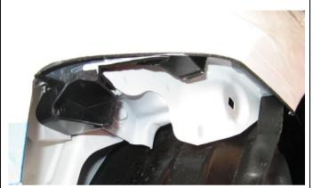
37. Refit the RH & LH bumper retaining brackets and secure them properly with the screws previously removed.
