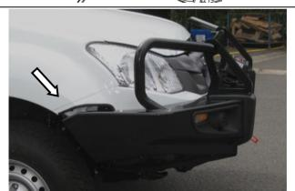
Position the bar so that the rear of the wing is parallel with the vehicle fender and lines up with the wheel arch. The nominal distance between the vehicle fender and the bull-bar is 48mm.
