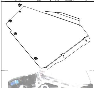
Fit the M6 cage nuts to the two wing stone guards (4 per stone guard).
