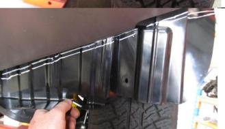
Remove the two wing stone guards and mark a second line 5mm above the first line on the RH and LH wheel liners
