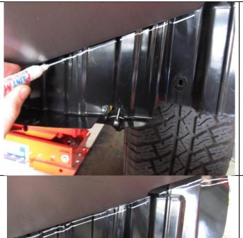
73. Loosely fit the RH and LH wing stone guards to the bull-bar. As shown on the adjacent photo, use a white marker to draw a line on the wheel liner at the lower rear edges of the stone guards.
