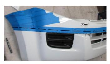
11. Cover the vehicle bumper bar with protective low tack tape in the regions where it is to be trimmed.
