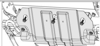
Refit the original vehicle stone guard using two of the original M10 bolts, at the rear of the stone guard, and three M10 x 30 black SEMS bolts at the front.
