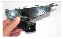
34. Use a hack saw to cut the RH and LH bumper retaining brackets. Once these cuts have been completed the parts should look like the adjacent images.
