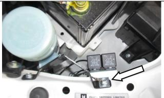
Undo the existing outer bolt holding the power steering reservoir bracket.
