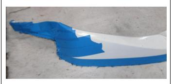
13. With the aid of an assistant, holding the bumper, trim and remove the lower portion of the bumper with an electric jigsaw.
