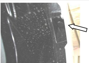
7. Remove and retain the upper rear bumper scrivets (1 per side).
