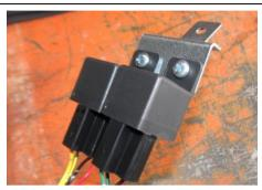
26. Attach the relays to the bracket supplied in the bull-bar fitting kit with two M5 x 12 pan head screws and two M5 nyloc nuts.
