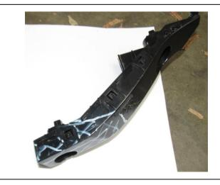
Use a white felt tipped pen to mark up the RH plastic bumper retaining bracket: the shaded region is to be cut off.
