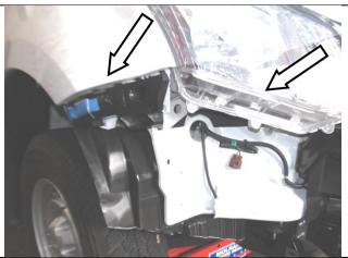
10. Carefully remove the bumper from the vehicle by pulling it away from the retaining clips located near the fenders and head lights.
