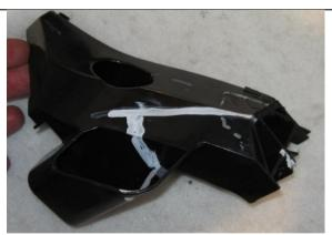
33. Remove the RH & LH bumper retaining brackets from the vehicle. Clearly mark the second cut lines on both sides of the parts as shown.
