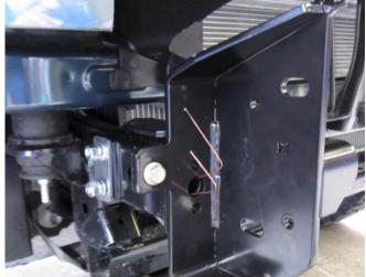
46. Re-use one of the chassis bolts, removed at step 15, to firmly locate the bull-bar mount bracket to the chassis.
