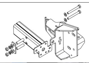
45. Loosely fit the right hand bull-bar mount to the chassis rail using the: M10 x 80 bolts (2 off), flat washers (4 off), crush tubes (2 off), rectangular plate (1 off), spring washers (2 off) and hex nuts (2 off) from the bull-bar fitting kit.
