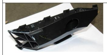
30. Use a hack saw to cut and remove the shaded portion of the bumper retaining bracket as shown in the adjacent image.
