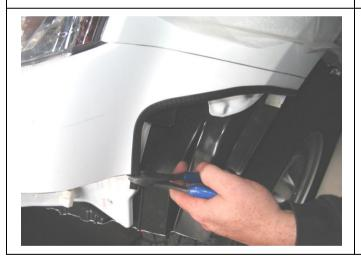
38. Fit the pinch weld, 2 off supplied with the bull-bar fitting kit, to the trimmed bumper as shown. Use side cutters to trim any excess pinch weld.
