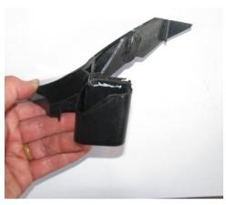
35. Use a white marker to mark the upper wheel liner rectangular cut-outs approximately 60mm high x 20mm deep as shown. Next, use a sharp utility knife to cut out these rectangles from the RH and LH wheel liners.
