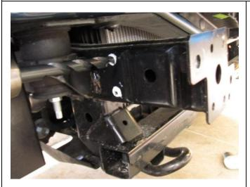
41. Drill two Ø13mm holes through the outer wall of the chassis rail only.
