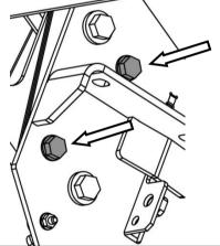
61. Once satisfied with the fitment of the bar to the vehicle, fit the M10 x 45 hex bolts to the RH & LH mounts (4 off - 2 per mount), flat washers (4 off) and flange nuts (4 off).
