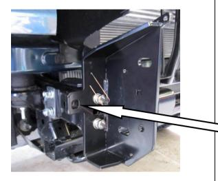
Fasten the two M10 x 30 SEMS bolts to the nut plate inserted in the chassis at step 44. Use the wire, shown in the adjacent image, to correctly position the nut plate.
