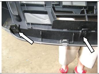
6. Use a flat head screw driver to unclip the vehicle grill from the bumper (4 places). Remove and retain the vehicle grill.
