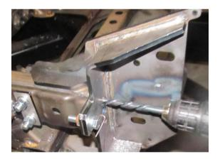
47. Use a punch to mark the two holes in the front of the chassis rail.
