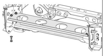
Loosely fit the centre bull-bar brace to the bull-bar mounts using four M10 x 25 hex bolts, four flat washers and four flange nuts are shown.
