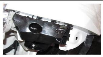
31. Loosely refit the LH and RH bumper retaining brackets. It is not necessary to screw them in place yet.
