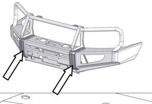
52. Attach the buffers to the bar as shown using twelve M6 flange nuts.
