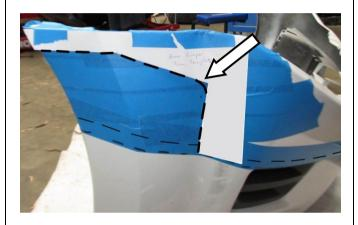
12. Cut the A3 paper template along identified cutting line (Part Number 3789124).
