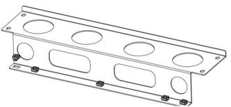
67. Fit five M10 cage nuts to the centre bull-bar brace.
