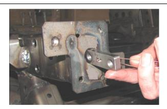
44. Insert the nut plate, from the bull-bar fitting kit, through the front flange of the chassis rail with the wire attached.
