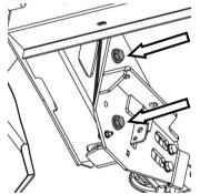
Use the M12 x 50 hex bolts (2 per mount), flat washers (4 per mount), spring washers (2 per mount) and hex nuts (2 per mount) to secure the bar.
