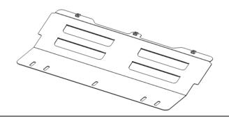
66. Fit three M6 cage nuts to the centre stone guard as shown.
