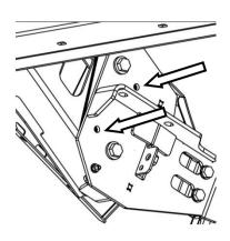
58. Once satisfied with the position of the bar on the vehicle drill the four Ø10mm pinning bolt holes (2 per mount).
