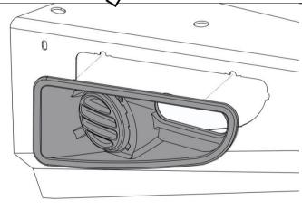
53. Assemble and install combination light surrounds (p/n 3163015) as per instructions no. 3786421 supplied with surround kit. Note: Optional fog lamps can be installed at this point as per fitting instruction no. 3783315 supplied with fog lamp kit no. 6821201.
