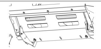
Fit the centre stone guard to the bull-bar / vehicle with: three M6 x 20 black hex bolts, spring washers, flat washers and two M10 x 30 black SEMS bolts.
