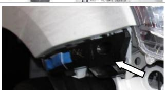
Carefully remove the RH and LH black plastic bumper retaining brackets. Keep the fastening screws as they will be reused.
