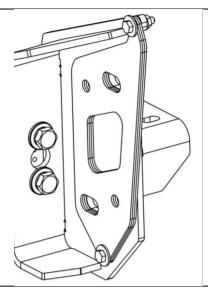
51. Fit an equal number of 2mm packers to the RH and LH mounts as required with the M6 x 25 bolts (2 per mount), flat washers and flange nuts.
