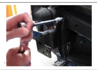
16. Unbolt the RH & LH bumper retaining brackets.
