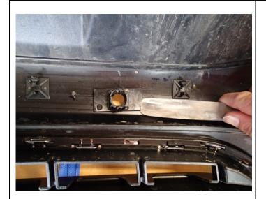
15. Using a paint scraper or something similar carefully remove parking sensor mount bracket from bumper making sure not to damage the bracket in the process.
