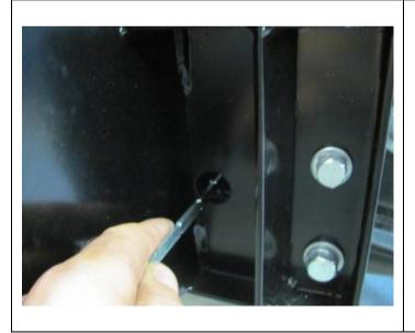
33. Using the supplied captive nut plate fit a M10 cage nut, using the access hole in the bull bar mount at the front of the chassis rail locate the cage nut behind the drilled hole and fix using M10 bolt and washer set.
