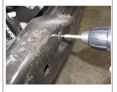
25. Remove the screws located on the VW bumper mount as shown in the figure.
