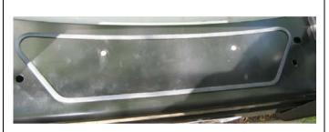
64. Fit panel to top face on bull bar using stainless steel 2 x M6 dome head screws and stainless steel flat washers and flange nuts.
