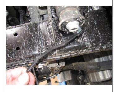
22. Fit two M8 cage nuts to the supplied captive nut plate as shown below, then slot the assembly through the access hole in the chassis, once in place loosely fix with the M8 bolt and washer set.
