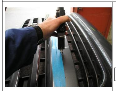
12. At this stage using an electric jig saw or a similar tool cut along the masked line which on the flare meets up with the 85 mm line (as indicated in step 7).
