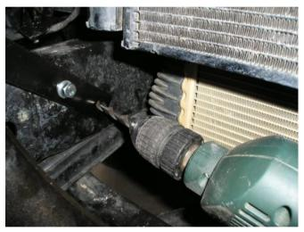
32. Now using the brace straps lower hole as a guide drill a 10 mm hole into the vehicles chassis rail
