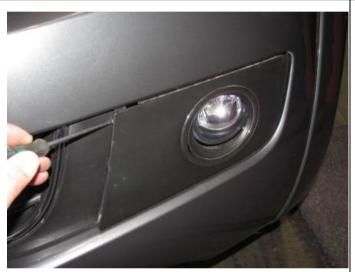
Remove the bumper from the vehicle by unclipping light covers to expose mounting bolts hidden behind, proceed to undo all required bolts.
