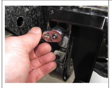
24. On the opposite side there are existing bolts which hold the factory sump guard in place loosen the bolts and place the stone tray bracket behind the factory bracket then tighten both sides of the stone tray bracket to the specified torque.
