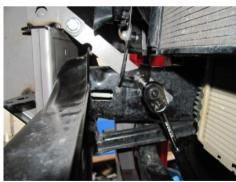
30. Remove the bolt retaining the VW horn bracket and place bull bar mount strap brace behind the bracket and secure using existing hardware
