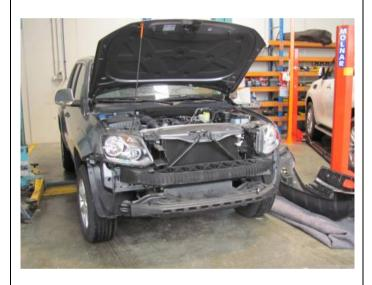
21. Remove the bumper reinforcing plastic and foam pads
