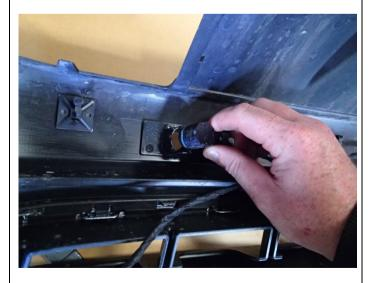
14. Cut cable ties holding the parking sensor loom to the bumper and remove loom and sensors.
