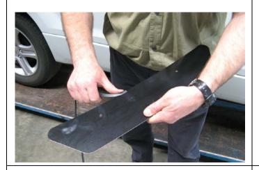
63. Apply rubber mould to edge of winch hole cover panel and trim off excess.
