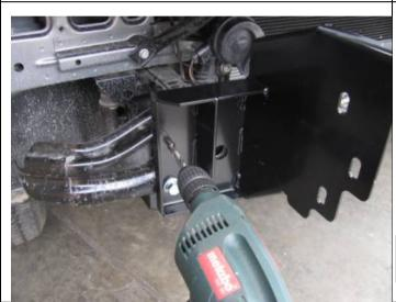
29. Once in place drill the remaining two holes using the guide holes in the bull bar mount with a 10mm drill bit, now that the holes are drilled secure the M10 bolt and washer sets on the drilled holes. All of the bolts may now be tightened to their specified torque.
