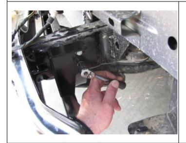
23. Place the stone tray bracket mount under the loose hardware.
