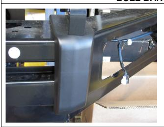
45. Fit the buffers to either side of the bull bar using 6 x M6 flange nuts. Do not over tighten.
