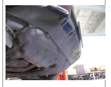
11. Undo the under body protection plate as well as the retaining bolts located in the wheel arches and above the grill, disconnect fog lamps and parking sensors if fitted then remove the bumper.
