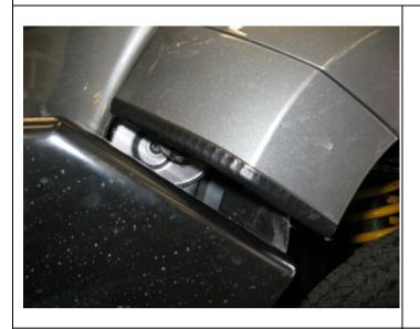
20. Fit pinch weld to cut area as shown, and trim to length.
