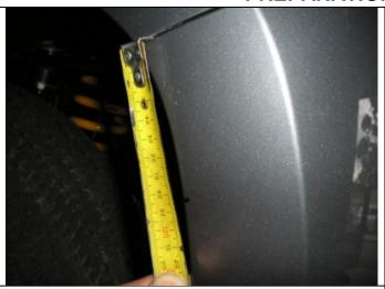
5. At this stage mark a point 85mm down from the panel edge on the flare.
