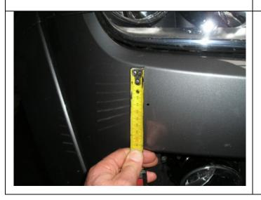
4. Continue to mark the bumper at small increments up until the corner of the light as shown at the same 50 mm measurement.
