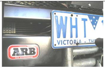
86. The licence plate can now be attached to the bull bar. Insert the two plastic square plugs supplied into the two square holes in the face of the bull bar (note slot allows for adjustable number plate hole pitch, ensure grommet flanges fit over the narrow width of the slot to engage correctly).
