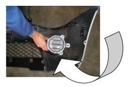
8. At this stage draw a point 120mm down from panel line on each side of vehicle and 20mm in the centre. (AS PER PHOTO) Using masking tape, join points to points across the front of the vehicle then remove bumper from vehicle. Using a jig saw or a small hand saw, cut across drawn line. Dress up with a file.
