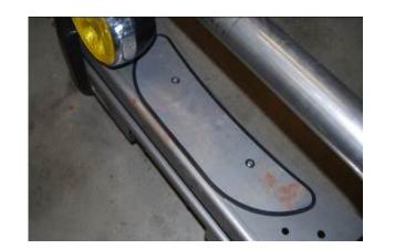
76. Fit rubber extrusion around the outer edge of cover panel if a winch is not going to be fitted to bar.
