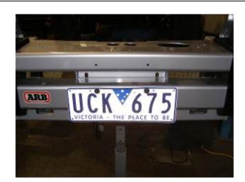
77. If you are not having a winch fitted to the bar, fit plastic grommets into the round holes and secure using black pan head screws to secure number plate to bar as per photo.
