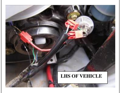
58. Pull indicator loom up into engine bay to scotch lok wiring onto vehicle indicator/clearance lamps
