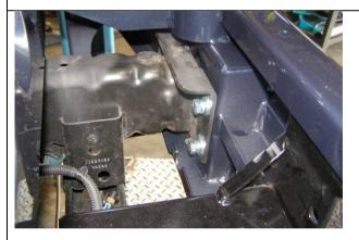
Loosely fasten bull bar to vehicle chassis using M10 fasteners supplied in chassis mounting kit.
