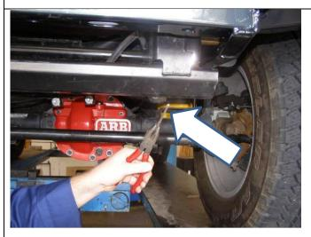
13. Tighten all chassis mounting fasteners to correct torque specifications listed on page 2.
