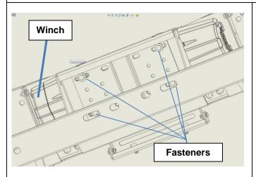
16. Lower winch onto bull bar mounting platform carefully aligning with slots.
