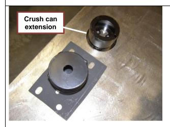
Attach crush can extensions supplied with bull bar to crush cans using 6x self-drilling screws supplied with crush can extension fitting kit ACCESSORY Part No 3550140 (3x screws per crush can).
