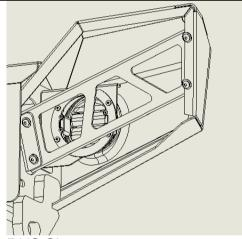
22. Fit wing braces to bull bar using M8 fasteners supplied with wing brace fitting kit.
