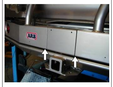
46. Align faces of centre cover panel with wheel carrier, jerry can carrier or cover panel and tighten securely.
