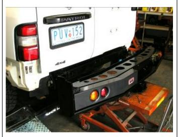
26. With the help of a friend fit bar to vehicle. (Rear bar shown with LHS cover panel fitted.)
