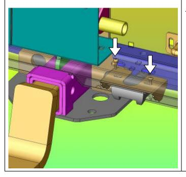
71. Fit trailer plug to recess using M5 pan head screws as shown by arrows.
