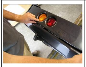
12. If a wheel carrier or jerry can carrier is not to be fitted a cover panel must be fitted.
