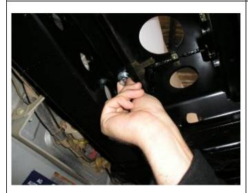
31. From underside of rear bar, fit **M10 x 35 bolt**, spring washer and flat washer to caged nut plate in crossmember.
