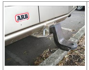
72. Fit gooseneck with pull pin and spring clip as shown.
