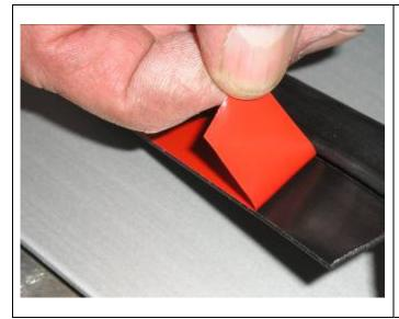
69. Carefully remove backing tape on the rubber strip and fit to step plate working from the centre outwards. Make sure rubber strip hugs the front and rear edge of the aluminium step plate.
