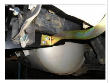
51. Using two **M8 x 25 bolts**, flat washers and flange nuts fit end surround braces to vehicle chassis. (RHS shown.)
