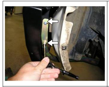
52. Using **M8 x 25 bolts**, flat washers and flange nuts secure end surrounds to braces finger tight. (RHS shown.)
