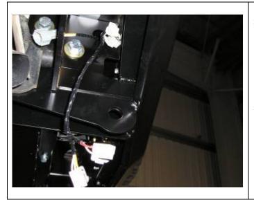
38. Feed loom through centre section of rear bar to outer ends of bar, through holes in top of side plates and connect to tail light assemblies and vehicle loom
