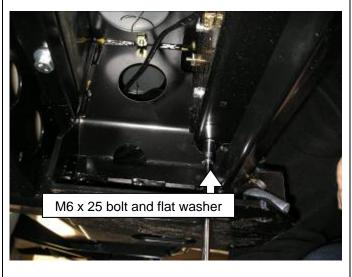
45. From underneath rear bar pass two **M6 x 25 bolts**, spring washers and flat washers through the aligned parts and finger tighten.
