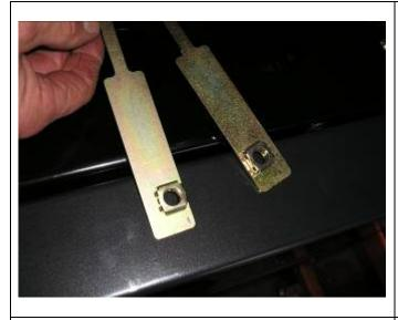
23. Fit M10 caged nuts to crossmember nut plates.
