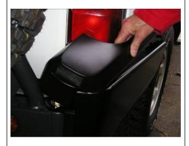
57. Fit urethane buffer to top of end surround using M6 nyloc nuts and large black flat washers.
