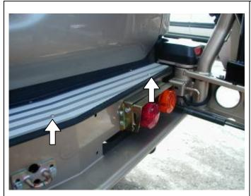
70. Using **M6 button head cap screws** fit aluminium step plate.
