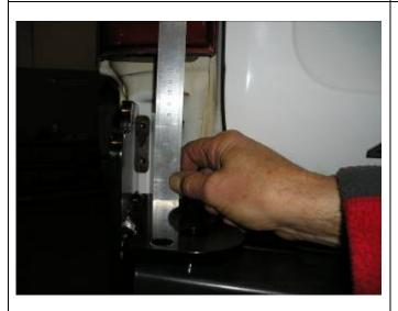
34. Take a measurement from the top of rear bar to underside of tail light to check if rear bar is level.
