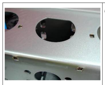
8. Fit M6 cage nuts (12 total) in square holes in top and front of bar as shown.
