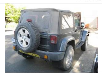
1. NOTE: To fit the ARB Rear Bar, the vehicles plastic inner guard liner must be cut. This is done at stage 4.
