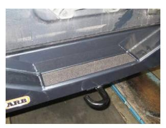
With the bar fitted to the vehicle, now apply the grip tape to the centre of the vehicle, making sure to align centrally
