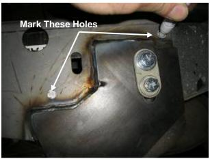
5. Now using 2 people, fit the bar to the vehicle. The chassis brackets slide either side and sit on top of the chassis rails
