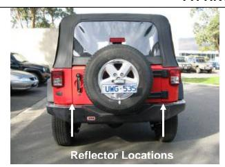
13. If the vehicle was originally fitted with reflectors in the bumper, then the reflectors provided in the fitting kit should be fitted to the vehicle in the location shown left.
