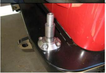
2. Place long shaft in centre M20 hole. Fit support hub over main shaft and line up the three M10 mounting points with holes in bar as shown in photo. Support may need to be tapped on using a soft hammer. Secure using M10 socket head cap screws and flange nuts. Secure main shaft under bar surface using M20 nyloc and flat washer.
