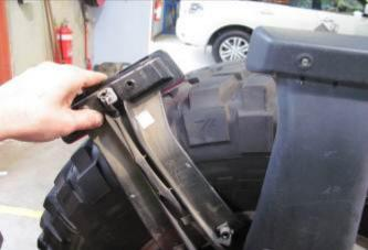
7. Remove JK wheel holder from vehicle and retain all components. Remove and un-plug stop light housing.
