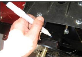
25. Move wheel mount inwards 20mm. This will place some load on the tyre when all is secured. Mark hole position, drill to 10mm and secure using M10 SEMS bolt and M10 flange nut. Tighten M10 bolt first followed by side bolts to specified torque.
