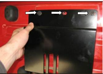
3. **FOR YJ-TJ.** Remove O.E tailgate bracket and stop light if fitted. Remove lower left bump stop from tailgate and plug hole using M6 bolt and flat washer. Retain bump stop for fitment to arm.
