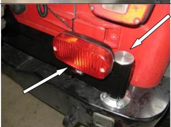
27. If fog light is fitted mount to new bracket on arm. Using a soft hammer fit hub cap to hub assembly.
