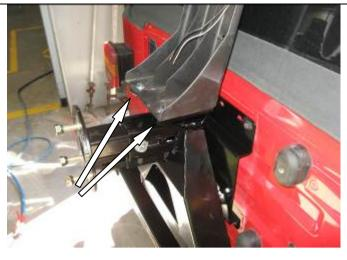
18. **YJ-TJ.** Place M8 cage nuts on bottom surface of light mount bracket. Secure stop light to bracket using four M8 x 20 bolts, spring washers and flat washers. Tighten all bolts to specified torque.
