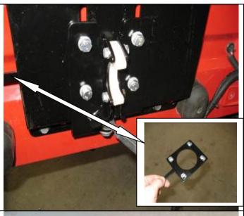
5. **YJ-TJ.** Install stop assembly to bracket as shown using M8 black bolts, flat washers and cage nuts in cage nut plate. Slide cage nut plate around the back of the bracket and secure finger tight.
