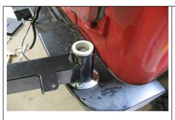
13. **ALL MODELS.** Smear a fine layer of bearing grease on all surfaces of bushes. Place bottom plastic bush in arm (tapered version) and place arm onto spindle. It may need a tap with a soft hammer. Place top bush (square shoulder) into arm by tapping with a soft hammer. Secure using M20 nyloc nut and flat washer. Set initial torque to 55Nm.
