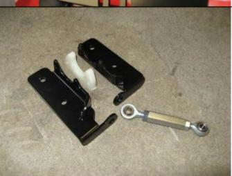
4. **ALL MODELS.** Lay out arm stop bracket and components as shown. Lubricate rod ends with 'CRC dry glide' or similar. Apply as per manufacturer's instructions. Fit M10 left and right thread nuts to rod ends before fitting to turnbuckle. Secure nylon block to brackets using two M6 x 30mm bolts, flat washers and M6 nyloc nuts. Secure rod end to brackets using M10 x 35 bolt, Spring washer, flat washer and flange nut.
