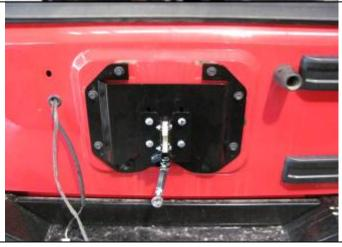
8. Install bracket to vehicle and tighten all bolts to specified torque.
