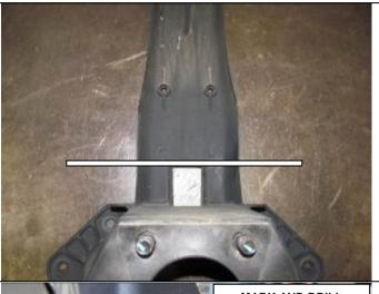
19. **JK.** Mark a line across the JK wheel mount as shown where the square access hole stops. Using a cutting disc or similar remove stop light section from mount. De-burr and paint surfaces.
