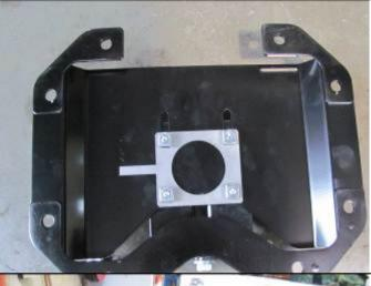
6. **JK.** Fit stop assembly to JK tailgate bracket as shown before fitting to vehicle.
