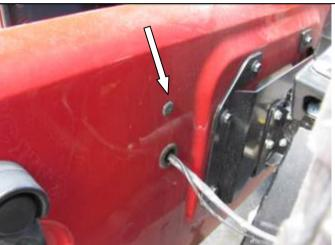
Clean area around holes in tailgate. Cover holes in tailgate using the two self-adhesive grommets.
