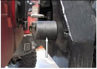
JK. Pull out the two rubber tyre rests from the JK tailgate and cut to a length of 50mm.
