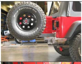
26. Mount spare tyre back to vehicle and check operation of arm. Due to varying weights of wheels and tyres it may be necessary to adjust nylon block position. Allow the arm to 'ramp up' on the Nylon block no more than 10mm. Test operation of arm. If more resistance is required tighten Nyloc nut on hub further, if less resistance is required back Nyloc off. The initial 55Nm or tighter is recommended as this will prevent arm and door swinging out too easily on steep angles.
