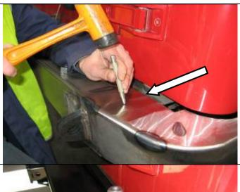
I. ALL MODELS. Locate laser cut circles on RH side of bar. Punch out using a centre punch. Clean any burrs and paint holes.
