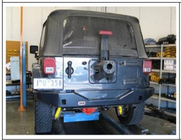
If vehicle is already fitted with ARB Rear Bar (Part No. 5650360) remove in reverse order of fitting instructions (Part No.3789186 stopping at step number 5). If ARB Rear Bar is not yet fitted carry out steps 1 – 5 from Fitting Instructions (Part No. 3789186).
