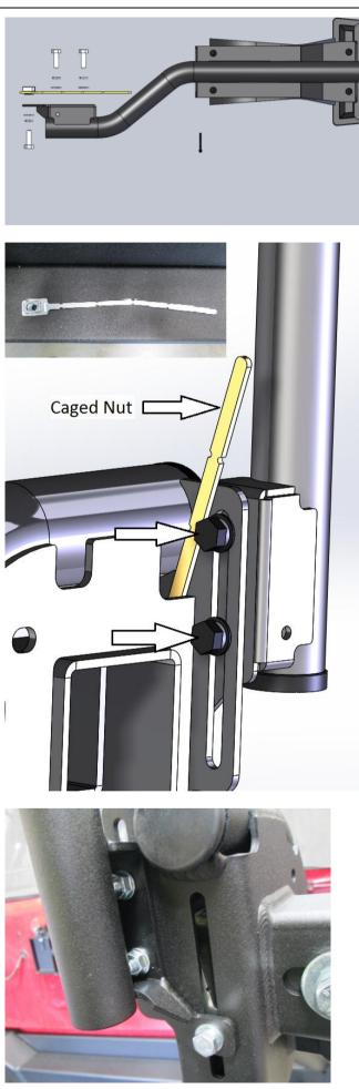
Mount Light Post to Carrier Arm. Use M8 x 25 Bolts, M8 Spring Washers, M8 Flat Washers, M8 Flange Nuts, M8 Cage Nut and Cage Nut Plate.
