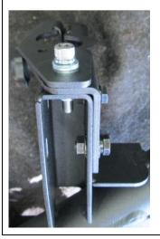
22. -Install Hi-Lift Locking Plate and M10 Knob. Use M8 x 40 S/Steel SHCS, M8 S/Steel Flat Washer and M8 NylocNut.
