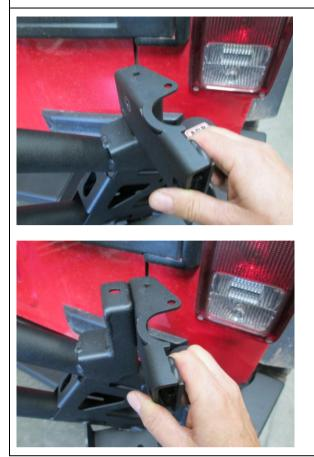
21. Install Hi-Lift bracket. Use Bolts M8 x 20, M8 Spring Washers, M8 Flat Washers and M8 Flange Nuts. Do not tighten fully.
