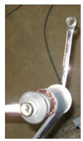
Fitting the bearing separator & puller again to push the bush in further so it is centrally located in the spring.
