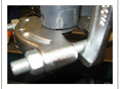
Using the bearing puller as shown, push out the bush. A light lubricant can be sprayed between the bush and the spring to assist removal.
