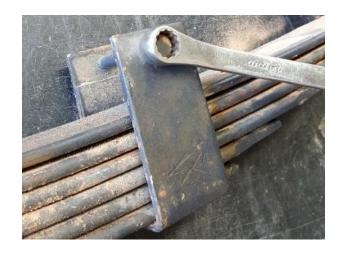
3. To disassemble the leaf spring ensure the spring is well secured with a clamp before releasing the centre spring bolt as shown. Use vice grips to secure the round head of the centre bolt if required.
