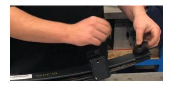
9. Fit the interleaf spacer plate supplied.
