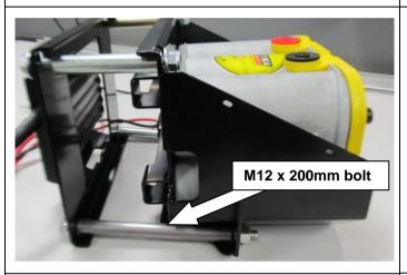
With the help of another person, Install the Battery tray using (3) M10 x 130 bolts and (1) M12 x200 bolt with washers under the heads and Nyloc nuts.
