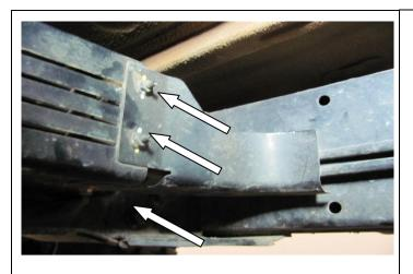
4. Vehicles with fuel line cooler, remove the corner guard, by unbolting the 3 M6 nuts.
