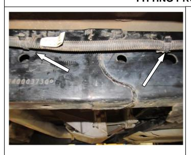
3. Unclip the Wiring Loom plugs from the Chassis on the outboard Drivers side.
