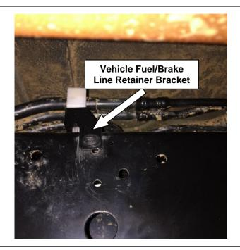
Fuel/Brake Line Retainer Clip Locate around bolt on chassis
