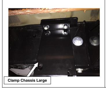
3. Locate the Fuel and Brake Line retainer bracket on the outboard passenger side of the chassis towards the rear of the car behind the centre body mount of the vehicle.
