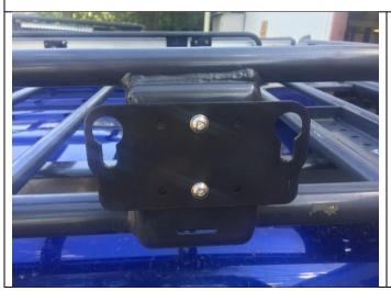
Place the mount plate onto the roof rack and attach using 2 x M6 x 25 setscrews and nyloc nuts into the previously drilled holes in the roof rack. Place washers under both the screw and nut.
