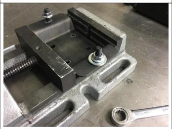
Place the bracket into a vice. Tighten the M8 nut against the washer to pull the knurled stud into the bracket.
