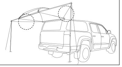
A: Push the press studs at either end of the side wall, into those at either end on side of the awning. Attach the velcro as shown. B: Attach the velcro tabs on the side wall around the support pole of the awning. C: Secure the bottom of the side wall by sliding a peg through the straps located in the bottom corners.
