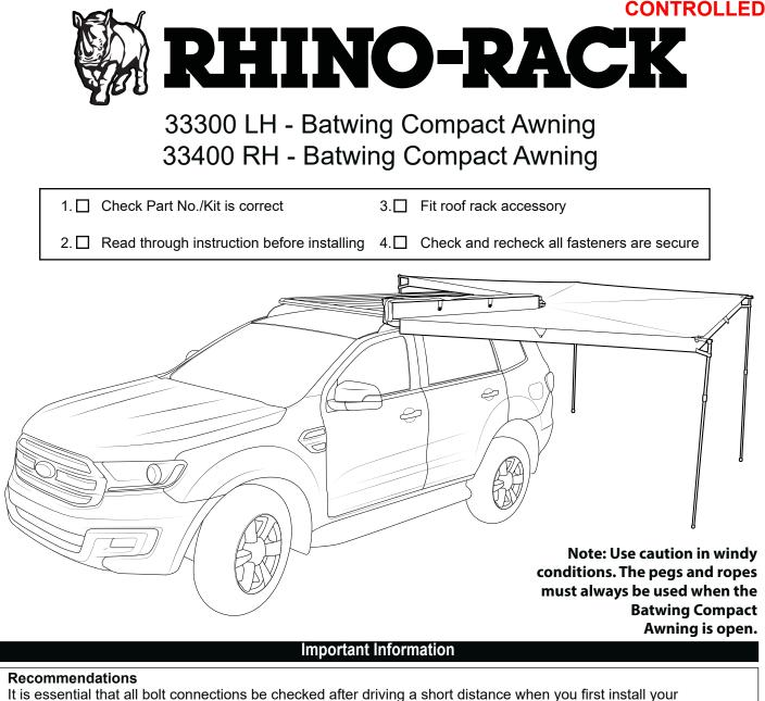
It is essential that all bolt connections be checked after driving a short distance when you first install your Rhino-Rack Batwing Compact Awning. Bolt connections should be checked again at regular intervals depending on road conditions, usage, loads and distances travelled. You should also check the roof bars each time they are refitted.
