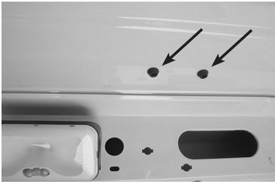
Locate the rubber plugs on the roof of the vehicle. Remove the rubber plugs by pushing them out through the top of the roof from inside the vehicle. Only remove the required amount of plugs for the amount of crossbars being fitted.
