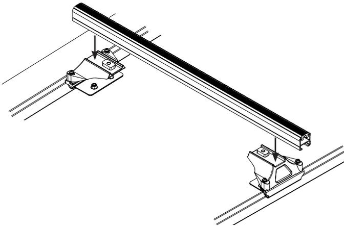
Place crossbars (Heavy Duty shown) onto the Legs. Lightly finger tighten the M10 bolt. Fasten the M6 x 35mm screws on the leg to 3-4 Nm (2-3 lb/ft) using the Torque Key supplied.
