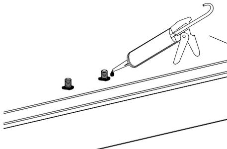
From on top of the roof apply Butyl Mastic sealer to the holes and around the protruding bolts on each of the inside brackets.
