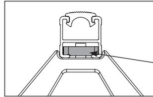
Channel nut must locate across the bar when tight.
