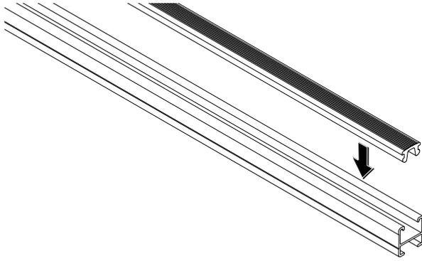
Insert a rubber buffer strip into the top of each crossbar.
