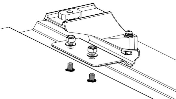
Carefully attach each external leg/bracket assembly to the protruding M8 bolts of the internal bracket using two of the M8 flat washers and M8 nyloc nuts. Tighten M8 nuts to 8-9 Nm (6-7 lb/ft).
