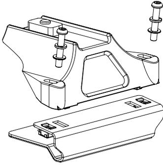
Prepare each leg/bracket assembly for installation using an M6 flat washer, M6 spring washer and M6 x 35mm screw on each side of the leg. Finger tighten only at this stage.
