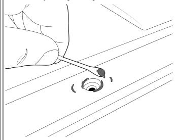
Apply Butyl Patches to **ALL** exposed threads. 1: Remove the backing tape from the Butyl Patch. 2: Place one patch over each exposed threaded hole. 3: Remove the backing from top of patches.
