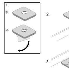
Fit the Rubber Bases from the QMFK04 kit to the RLT600 Quick Mount Bases.
