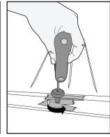
**Hex Head Screws:**Use a \*\*13/16 or 21mm socket wrench to remove the hex head roof plugs. Be carefull not to damage the plastic hex head while removing.
