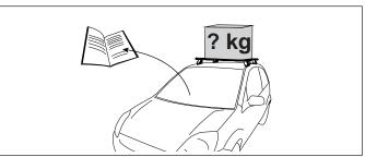
When these roof racks are to be used on a vehicle that is driven off sealed roads, the manufacturer maximum roof load rating (to be found in the vehicles User Manual) should be *divided by 1.5*. Do not forget to subtract the complete crossbar system weight from your maximum carrying capacity.
