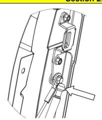
2.1) Use the same procedure as mentioned in section 1 for the LH side components except to place the narrower body strut onto the ball studs (4590022 for DMax or 4590025 for Colorado). This strut is a damper and it's piston can be moved in and out by hand to help with alignment. Ensure fasteners on LH side are torqued to 22Nm.
