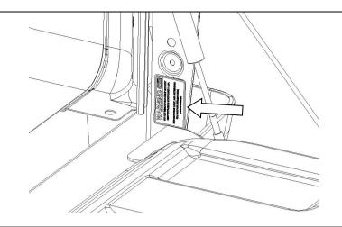
1.8) Fit warning label to vehicle tub as shown in the image. Onto the RHS. It must be fitted to the larger spring assist side and placed just below the lower tail light screw position.
