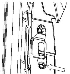
1.1) Using a 12mm socket remove the lower M8 bolt on striker bracket. Retain bolt.
