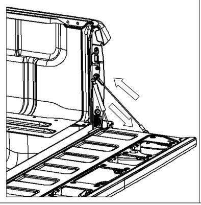
2.2) When complete open and close the tailgate to ensure correct operation. Make sure there is no binding or cables protruding.
