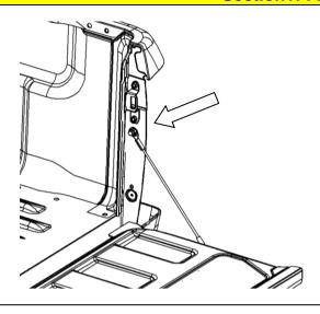
1.0) Remove existing cable and upper bolt assembly from the tub using 13mm socket and retain complete assembly. The cable can be left dangling from the remaining bolt.
