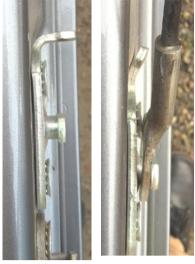
1.3) If the tailgate is fitted with cables, the tailgate retainer will have a bent tang on the lower side of it. Remove the retainer and straighten the tang so that it follows the line of the panelwork.
