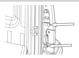
1.4) Place mounting bracket (3750331R) over the lower striker mounting hole and loosely fasten using the original bolt. Align the lower hole with the vacant 8mm hole in the quarter panel. Secure using the 16mm long M8 button head screw (6151874) and M8 flange nut (6151548) inside the tail light cavity. When complete tighten fasteners to 22Nm.
