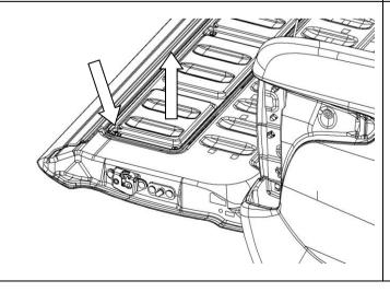
1.6) Remove the tailgate liner if fitted. Remove the screws securing the tailgate access panel and retain. Lift off and remove the access panel. Place it in a safe location for re-fitment at a later stage.
