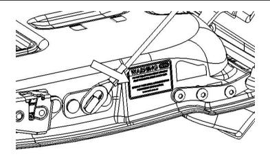
2.4) Fit warning label to vehicle tub as shown in the image. It must be fitted to the larger spring assist side and placed on the side of the tailgate as shown.
