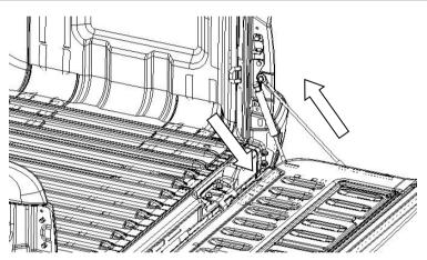
2.3) When complete open and close the tailgate to ensure correct operation. Make sure there is no binding, cables protruding or contact of struts to the vehicle tailgate or body of the vehicle.
