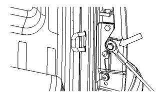
**1.5)** 4746010 Kit: Using the bolt and washers removed in step 1.1) attach the new cable to the quarter panel, keeping the washers in the same order as removed.
