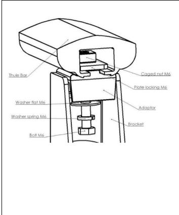
Fit locking plates to the carrier brackets using the M6 bolts, M6 spring washers, and M6 flat washers. Leave the fittings loose.
